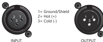
Balanced use of XLR connectors
